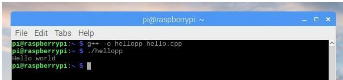
The screenshot shows a terminal window titled "pi@raspberrypi: ~". The window has a menu bar with "File", "Edit", "Tabs", and "Help". The terminal output is as follows:
