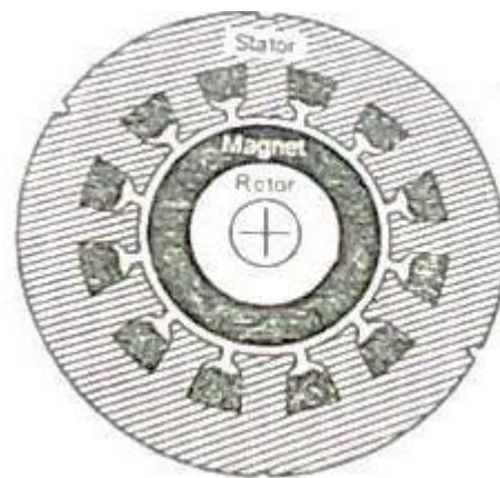
Figure 2.1.1 construction of BLPMDC motor
