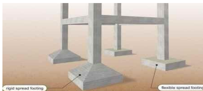
Fig 5: Flexible and Rigid Footings of a Structure
