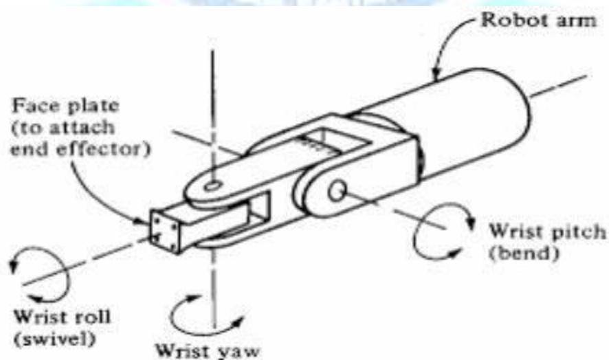
Wrist movement is designed to enable the robot to orient the end effector properly with respect to the task being performed. To solve the orientation problem, the wrist is provided with up to three degrees of freedom.
