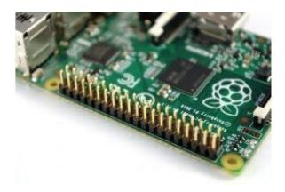
A GPIO pin set to output can provide either 3.3 volts, known as a HIGH signal, or 0 volts, known as a LOW signal. When set to input, it can read these same voltages.
