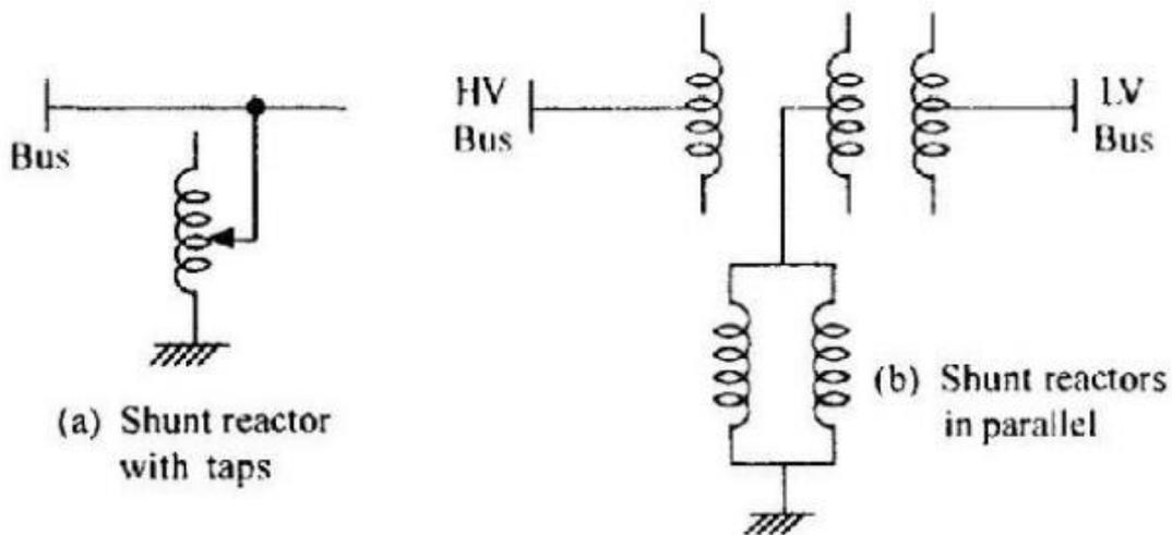
*Figure - Typical Shunt Reactor*
