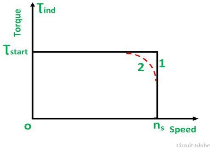
Curve 1 is the ideal curve, and the curve 2 is the practical hysteresis motor curve. The torque-speed characteristic of the hysteresis motor is different from an induction motor. Since, at the synchronous speed, the torque developed by an induction motor becomes zero, whereas in the hysteresis motor the torque is constant at all the speed even at the synchronous speed. Thus, from the curve, it is seen that the locked rotor, starting and pull out torque is equal.
