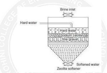
• Zeolite process results in *Zero hardness* – not suitable for public supplies – small amount is processed and mixed with un softened water to obtain standard limits.
