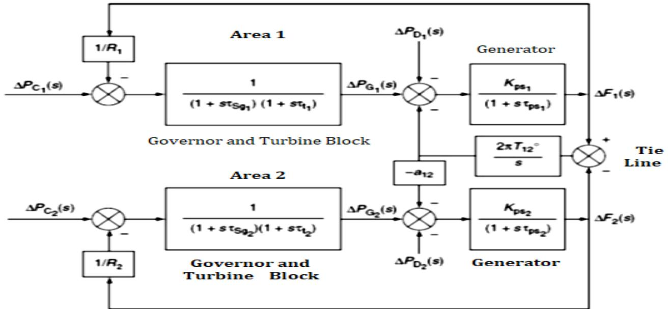
From the block diagram write the 's domain' equations
