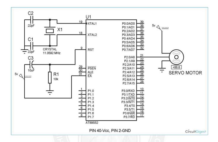
The position sensor senses the location of the shaft from its fixed position and sends the information to the control circuit. The control circuit decodes the signals accordingly from the position sensor and compares the actual location of the motors with the preferred position and accordingly controls the direction of rotation of the DC motor to get the necessary position. Generally the servo motor requires 4.8V to 6 V DC supply.
