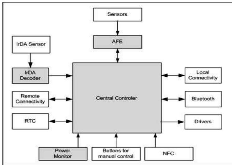
The Central Control Unit is the hub and brain of a home automation system. Common features of a central control unit are:
