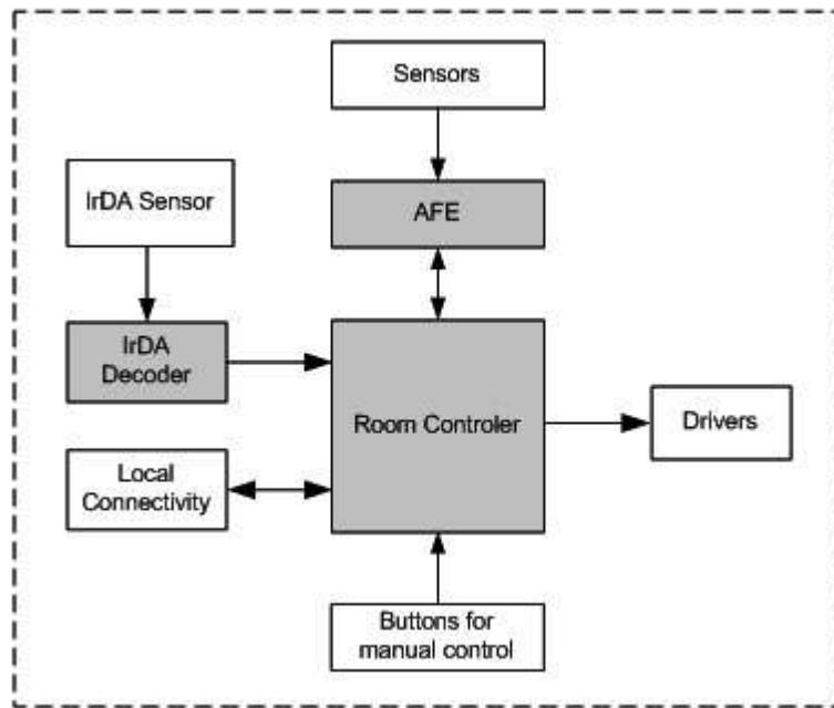
A Room Control Unit controls the appliances in a particular room. It has a set of sensors to sense the surrounding environment. Based on the current conditions, it can decide upon a course of action. Common features of a room control unit are:
