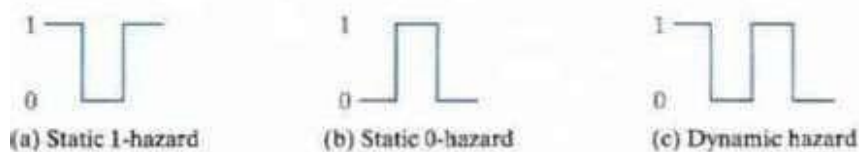
Fig 4.1 – Static and Dynamic Hazard
