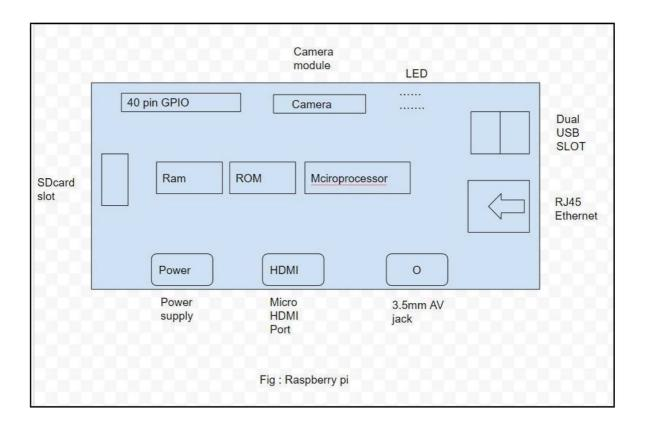
**Specs of the Computer:** – The computer has a quad-core ARM processor that doesn't support the same instruction as an X86 desktop CPU. It has 1GB of RAM, One HDMI port, four USB ports, one Ethernet connection, Micro SD slot for storage, one combined 3.5mm audio/videoport, and a Bluetooth connection. It has got a series of input and output pins that are used for making projects like – home security camera, encrypted door lock, etc.
