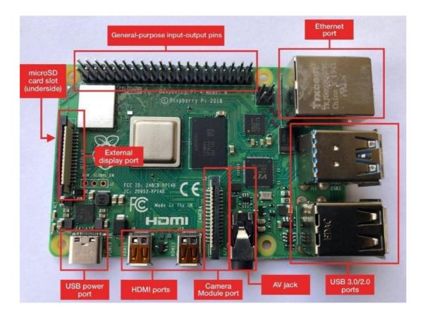
The Raspberry Pi 4 board contains the following components:
