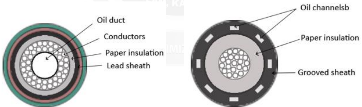
(i) Conductor channel
