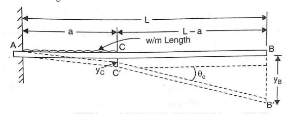
The beam will bend only between A and C, but from C to B it will remain straight since B.M. between C and B is zero. The deflected shape of the cantilever is shown by AC'B' in which portion C'B' is straight.
