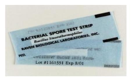
❖ Bls are critical for validating sterilization of equipment used in vaccine production (e.g., bioreactors, filling needles) and ensuring sterile conditions during aseptic processing, where terminal sterilization isn't always feasible (e.g., spray-dried vaccines).
