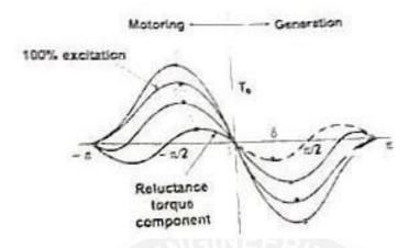
Figure 5.3.2 Torque Angle characteristics of salient pole [Source: "special electric machines" by Srinivasan page:1.3]
