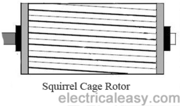
Most of the induction motors (upto 90%) are of squirrel cage type. **Squirrel cage type rotor** has very simple and almost indestructible construction. This type of rotor consist of a cylindrical laminated core, having parallel slots on it. These parallel slots carry rotor conductors. In this type of rotor, heavy bars of copper, aluminum or alloys are used as rotor conductors instead of wires. Rotor slots are slightly skewed to achieve following advantages -
