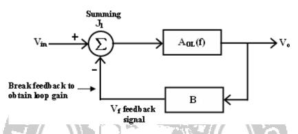
The block between the output and input is referred to as forward block and the block between the output signal and f/b signal is referred to as feedback block. The content of each block is referred -Transfer frequency' From fig we represented it by AoL (f) which is given by
