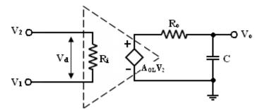
There is one pole due to  $R_0$  C and one -20dB/decade. The open loop voltage gain of an op-amp with only one corner frequency is obtained from above fig.
