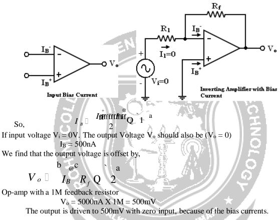
In application where the signal levels are measured in mV, this is totally unacceptable. This can be compensated. Where a compensation resistor  $R_{comp}$  has been added between the non-inverting input terminal and ground as shown in the figure below.
