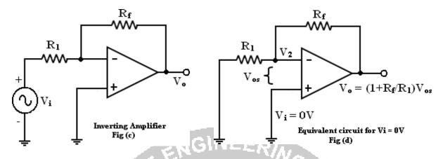
Let us determine the  $V_{os}$  on the output of inverting and non- inverting amplifier. If  $V_i = 0$  (Fig (b) and (c)) become the same as in figure (d).
