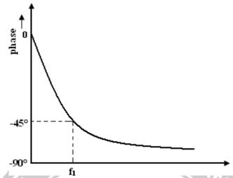
From the phase characteristics that the phase angle is zero at frequency f=0.
