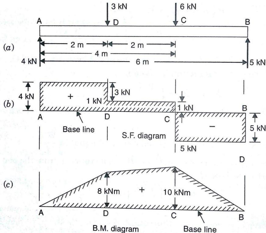
**BendingmomentCalculation:** [Sumof(VerticalforcexDistanceofloadactingfromrequired section)]
