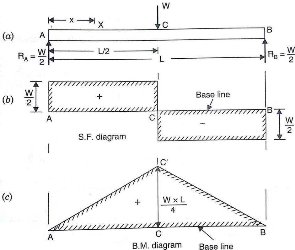
First to find the reaction force at A and B as \$R\_A\$ and \$R\_B\$ by the two steps are followed.
