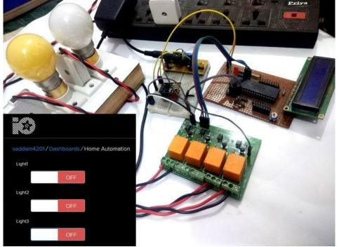
IoT based Web controlled Home Automation using PIC Microcontroller and Adafruit IO
