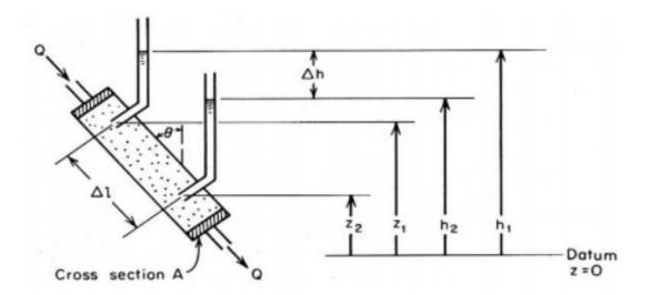
When water is introduced to the inlet channels of cylinderical pipe and allowed to flow through the porous medium, then it will take some time to get all pores filled with water and to attain flow rate equilibrium at inlet and outlet point.
