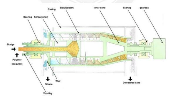
The bow spins at high speed which simultaneously separates water from the solids. The separated solids are compacted against the bowl wall, as shown in the figure. The solids are then conveyed to the centrifuges drying stage and the liquid separated is discharged continuously over the weir arrangements around the sides of the bowl.
