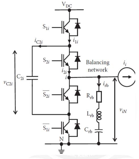
Fig 4.4.1 Three-level FCMC with balancing network
