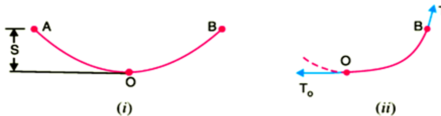
Figure 3.1 Sag in Overhead lines
