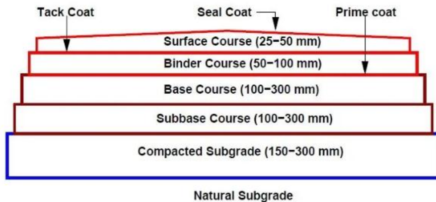
Figure 1.2: Typical cross section of a flexible pavement
