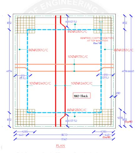
Reinforcement Detail of Two way Restrained slab
