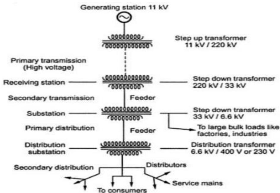
The power system is the complex enterprise that may be subdivided into the following sub-systems. The subsystems of the power system are explained below in details
