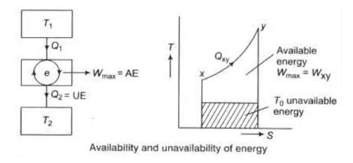
$$W_{\text{max}} = AE = Q_{xy} - T_0(S_y - S_x)$$
