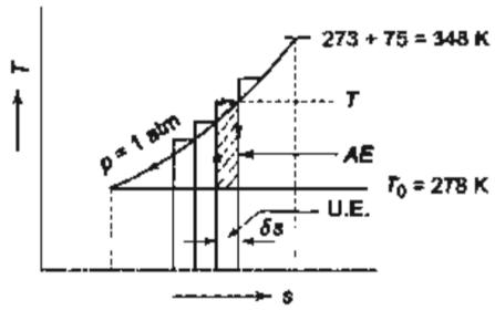
$$W_{\text{(max)}} = \text{A.E.} = -\lim_{348} \frac{278}{40} c_p \left(1 - \frac{T_0}{T}\right) \delta T$$
