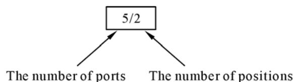
include 2/2, 3/2, 5/2, etc. The first number represents the number of ports; the second number represents the number of positions. A directional control valve that has two ports and five positions can be represented by the drawing in Fig. 8, as well as its own unique pneumatic symbol.
