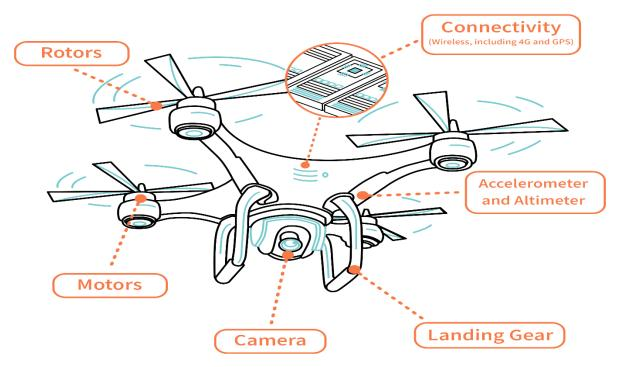
Here is an overview of the **main parts of a drone**:
