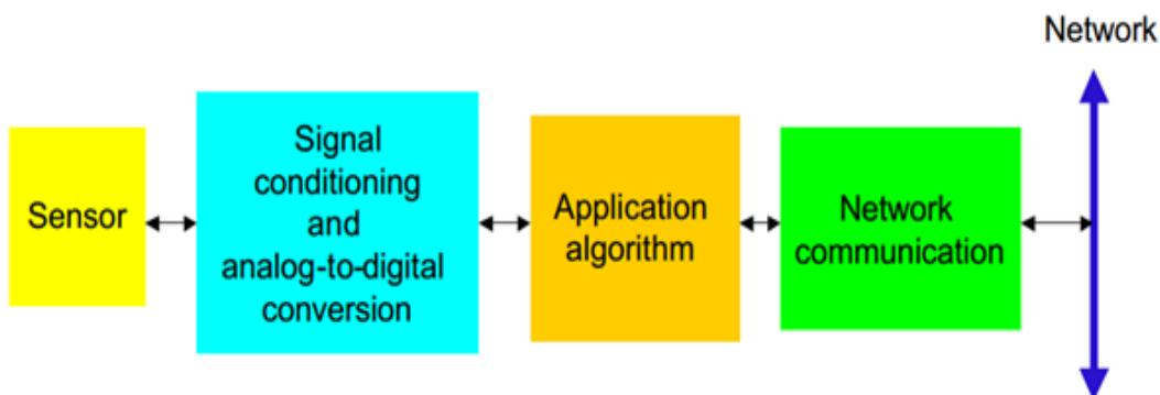
The sensor collects raw data from the environment. The raw signal from the sensor is often weak or analog. Cleans and strengthens the signal (signal conditioning) Converts analog signal to digital (ADC) so that electronics can understand it Application algorithm processes the digital data and makes decisions. After processing, the information is sent to another device or system through a network.
