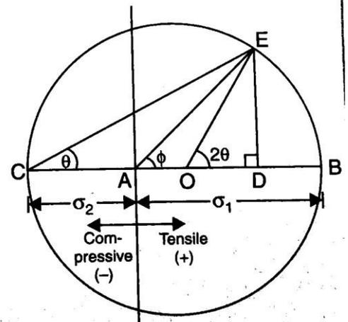
A body subjected to two mutually perpendicular principal tensile stresses with simple shear stress
