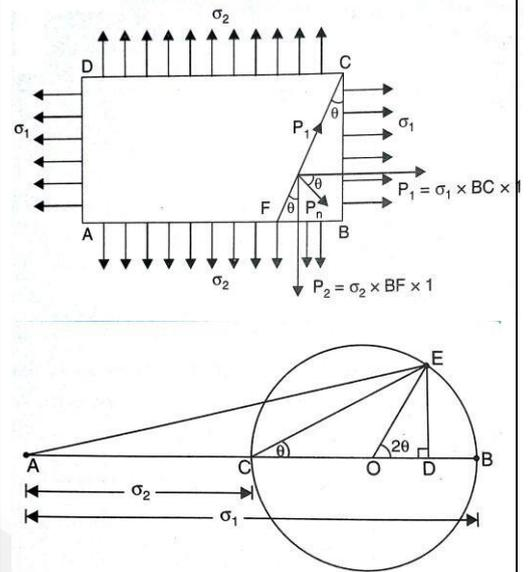
A body subjected to two mutually perpendicular principal tensile stresses which are unlike (Tensile and compressive)
