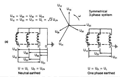
Voltage relationships of some systems currently in use and diagrams showing the arrangements and connections of the secondary windings of the in feeding transformers. The heavy broken lines represent the magnetic cores
