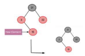
15 is inserted to the right of 3 and colored as red. Two red nodes are not possible and as the uncle node is red, change the color of parent and uncle as black.
