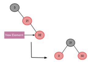
32 is inserted to the right of 21 and colored as red. Two red nodes are not possible so it needs a RR Rotation and we need to recolor to balance the tree. After rotating 21 becomes the root node which is red. But a root node cannot be red, So we need to recolor it as black. And 3 is the grandparent of 32 and hence recolor it as red.
