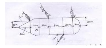
(ii) Determine a single equivalent force and its location along the longitudinal axis of the ship
