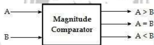
Fig : 2.21 - Block diagram of magnitude comparator
