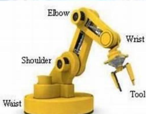
Robot anatomy is concerned with physical construction of the body, arm and wrist of the machine. Most Robots used in plants today are mounted on a base fastened on the floor.
