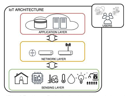
Three-layer Internet of Things (IoT) architecture. The data is collected through the sensing layer and transferred over the network layer to servers and databases in the application layer. Users connect to the system over the cloud.
